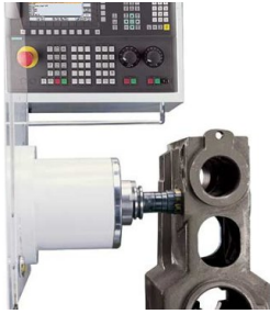
Multi-sided machining in one clamping
