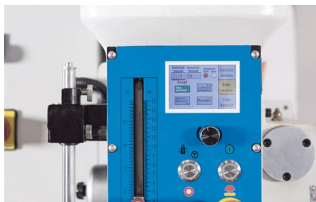
Modern operating concept with rugged touchscreen display
