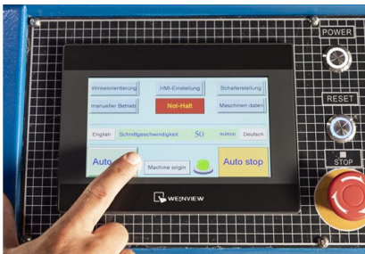
In Auto Mode, feed distance, cut angle, and number of cuts can be programmed within the respective configurations
