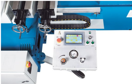
Manual saw frame angle adjustment with hydraulic drive (15°, 30° and 45°)
