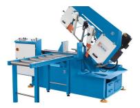
Hydraulic part clamping Coolant system Linear stop Feed roller table 1,2 m Operator manual
