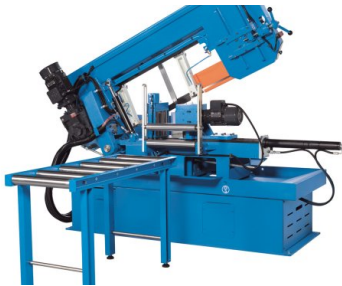
A feed roller table is part of the standard equipment package
