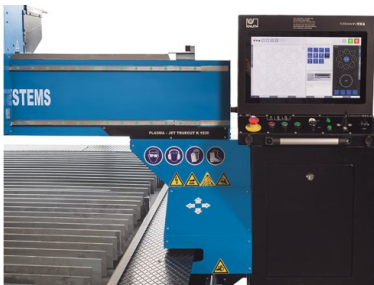
Powerful Eckelmann CNC-Unit with 19" touchscreen by ELO
