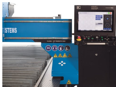
Powerful Eckelmann CNC-Unit with 19" touchscreen by ELO
