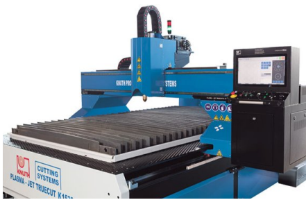
Dual-drive bridge design with dynamic AC servo drives on all axes
