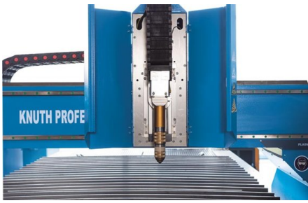
Quick-coupling for cutter head
