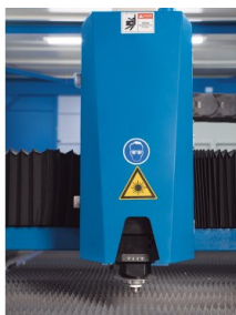
Smart cutter heads of the BLT 6 series also were custom designed for high-power laser cutting systems with max. 40 kW power
