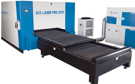
An automatic changer table system minimizes down-times by allowing simultaneous loading and unloading of the table during the cutting process
