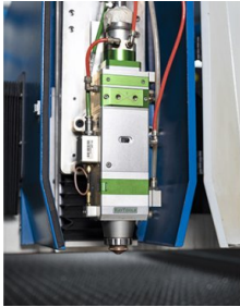
High-quality cutter head with auto-focus made by the RayTools
