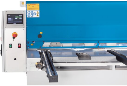
Lateral stop with scale and manually adjustable kerf setting
