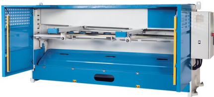
Lateral stop with scale and manually adjustable kerf setting
