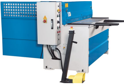
Back gauge is protected via sturdy enclosure and light curtain
