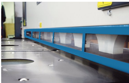
Material support rollers are recessed in the table for easy workpiece handling
