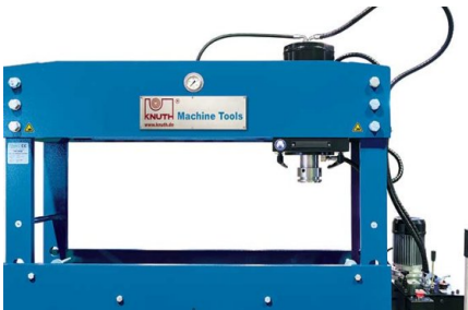
The hydraulic cylinder can be moved laterally and is clamped mechanically
