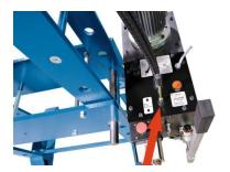
The press is operated via joystick
