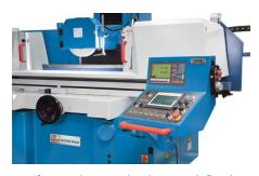
If set to Auto mode, the user-defined roughing and finishing parameters, number of spark-out strokes, and return to zero are automatically processed
