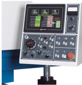
Touchscreen display for easy programming of grinding cycles
