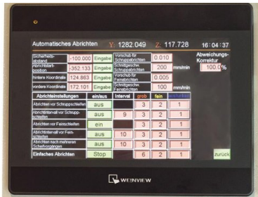
Dressing mode for grinding wheels with automatic dimension and speed (rpm) compensation ensures constant grinding rate and can be entered while in auto mode
