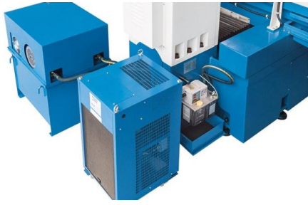
External hydraulic unit and oil cooler ensure thermal stability during continuous operation
