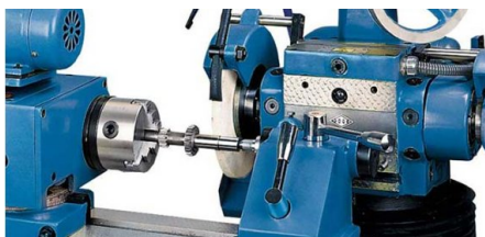
Outside cylindrical grinding for length up to 400 mm
