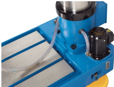
Large throat and work table that swivels and rotates
