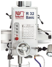
Hand-lever for quill feed is used to control the automatic feed
