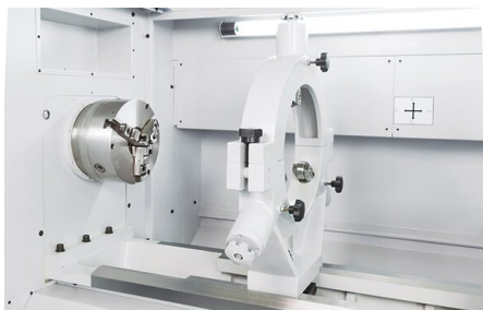
Option: steady rests up to 400 mm diameter
