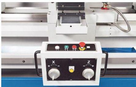
Compact control unit with electronic hand-wheels
