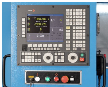
Compact control unit with electronic hand-wheels
