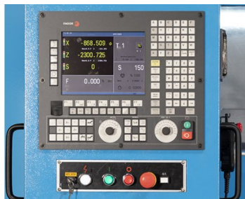
Compact control unit with electronic hand-wheels
