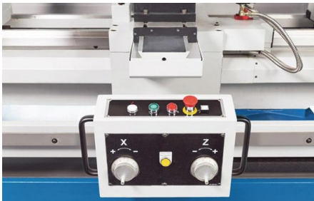
Compact control unit with electronic hand-wheels
