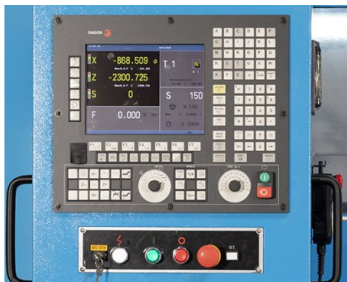
Compact control unit with electronic hand-wheels
