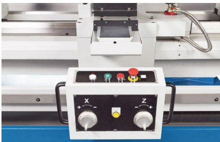
Compact control unit with electronic hand-wheels
