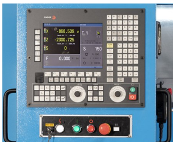
Compact control unit with electronic hand-wheels
