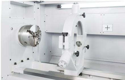
Option: steady rests up to 400 mm diameter
